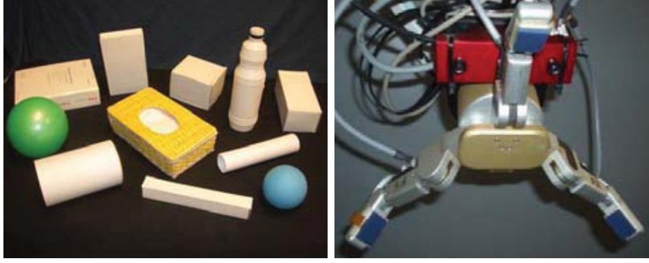
Figure 8.5: Left: Objects used for the experiments on black background. Right: Robotic setup consisting of a PA10-7C manipulator with a Barrett Hand and a Videre Stereo vision system.
